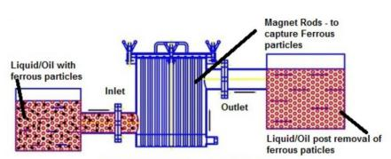
Liquid In Line Magnetic Separator
