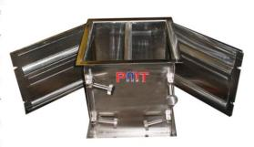
powerful magnetic circuit inside the chute. They are installed within the vertical gravity feed chutes for the extraction of iron particles from the product flow. As material enters through the box inlet, it passes over a centre deflector which angles the product flow towards the powerful magnetic doors. The iron particles in the product flow is then arrested and held by the powerful magnetic doors and the clean material passes through the box outlet.
